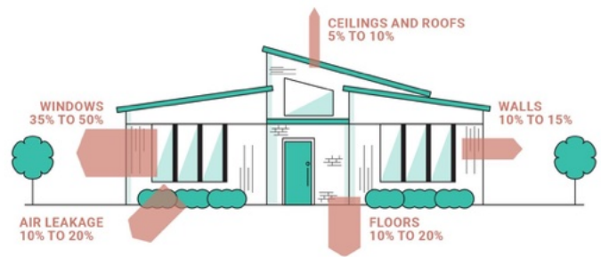
Typical heat losses in the winter for a standalone home insulated to the previous requirements.
